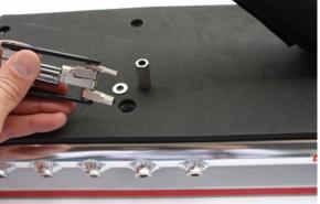
Be sure that all nuts connected to the boards are tight. Put the plastic caps to cover the holes.
