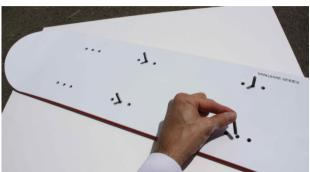
Put the rubber cylinders over the hexagonal insert bolts. If done once, you can install the foam pads (optional) as shown under the frame.
