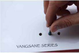
Put the rubber cylinders over the hexagonal insert bolts. If done once, you can install the foam pads (optional) as shown under the fork. Tighten the fork with 4 washers and 4 lock nuts. After it, the fork needs to be centralized on the front board.
